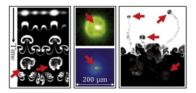
Left: evolution of a multimode shocked fluid layer experiment. Middle: experimental (top) and simulated (bottom) x-ray self-emission during an ICF capsule implosion. Right: volume fraction from RMI simulations. Red arrows indicate likely vortex rings and dipoles. All images are reproduced with permission. Credit: *Physical Review Letters* (2023). DOI: 10.1103/PhysRevLett.130.194001
