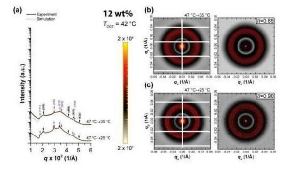
Experimental and simulated (a) 1D- and (b-c) 2D-SAXS patterns of the 12 wt% PBPEO solution by temperature-quenching from disordered states to the crystallization temperatures noted. The left panels of the 2D-SAXS are experimental, and the right panels are simulated patterns. Credit: *Soft Matter* (2023). DOI: 10.1039/D3SM00199G
