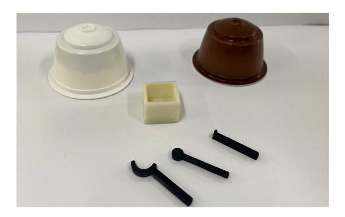
Used pods and examples of parts produced by 3D printing, also called additive manufacturing. Credit: Bruno Campos Janegitz/UFSCar
