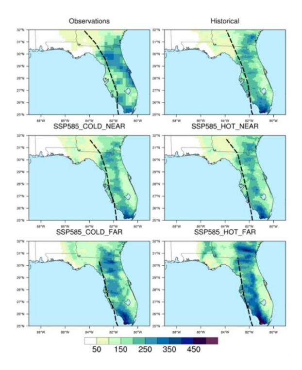
A TGW simulation shows precipitation due to Hurricane Irma under four future scenarios, including historically simulated precipitation and observations. Credit: U.S. Department of Energy
