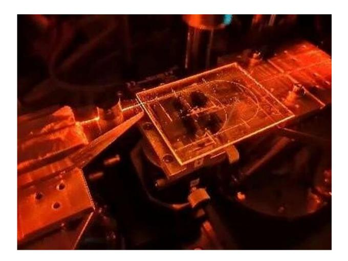
The silica-based QKD receiver shown consists of a photonic integrated circuit and two external single-photon detectors. Credit: Simone Atzeni, CNR-IFN
