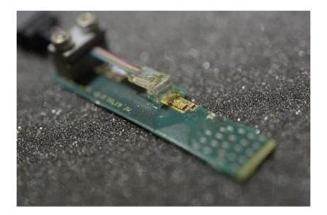
Researchers have developed a quantum key distribution (QKD) system based on silicon photonics that can transmit secure keys at unprecedented speeds. The QKD transmitter (pictured) combines a photonic and electric integrated circuit with an external diode laser. Credit: Rebecka Sax, University of Geneva
