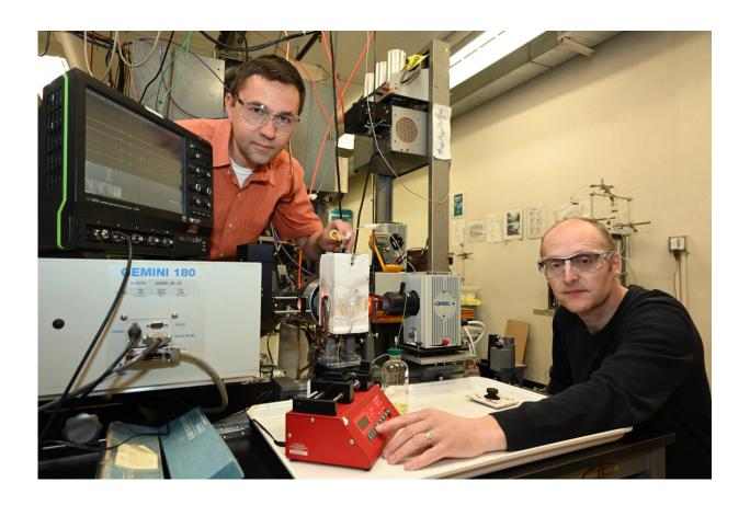
Dmitry Polyansky (left) and David Grills in the pulse radiolysis lab where the research was conducted. Here, Grills programs a syringe pump that delivers the catalyst to the radiolysis cell. Polyansky adjusts the radiolysis cell inside a white insulated compartment. Credit: Brookhaven National Laboratory
