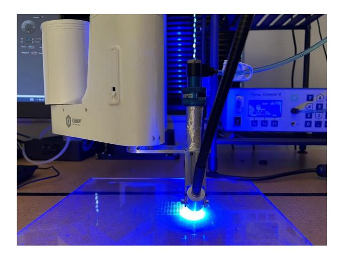
NC State researchers demonstrated that it's possible to make carbon dioxide capture filters using 3D printing. Credit: Sen Zhang and Jialong Shen, NC State.
