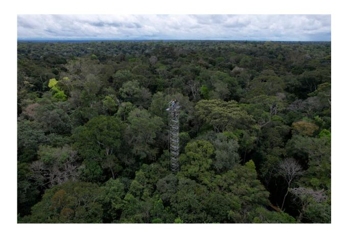
Workers appear on a tower that will be part of a complex of towers arrayed in six rings to spray carbon dioxide into the rainforest north of Manaus, Brazil, on Tuesday, May 23, 2023. Each ring will consist of 16 aluminum towers as high as a 12-story building. The aim is to understand how the world's largest tropical forest responds to climate change. Credit: AP Photo/Fernando Crispim
