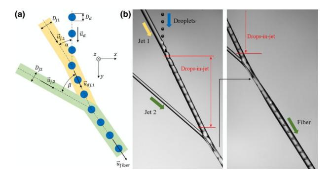
(a) Kinetic and geometric parameters relevant for the production of fibers with regular inclusions. (b) Pictures of the collisions observed in the collision plane. The collisions between the droplets and jet<sub>1</sub> enable the formation of the liquid drops-in-jet structure, which subsequently solidifies thanks to the supply of cations ensured by the collision with jet<sub>2</sub>. Credit: *Physical Review Applied* (2023). DOI: 10.1103/PhysRevApplied.19.054006
