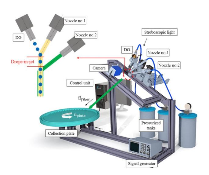
Schematic illustration of the experimental setup (prototype) designed for the production of advanced fibers. (Left) Zoom into the two subsequent collisions respectively involving droplets (blue) and jet<sub>1</sub> (yellow), and the drops-in-jet structure with jet<sub>2</sub> (green). (Right) Overview of the various components enabling
