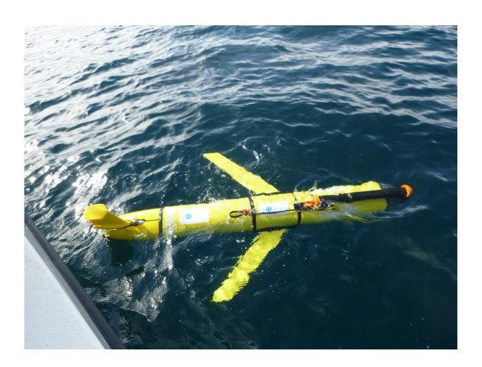
Scientists used ocean gliders to collect data, including temperature, salinity and nutrient levels in Storm Bay. Credit: CSIRO
