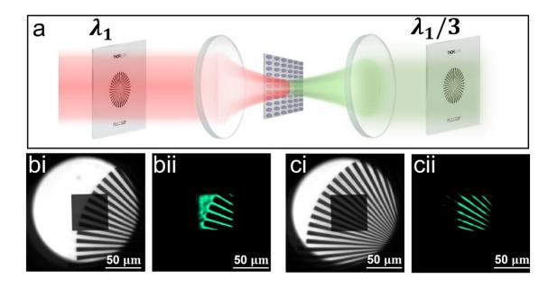
(a). The schematic of THG imaging based on Si membrane metasurfaces. (bi and ci) The images of a Sector Star Target and the metasurfaces under white light source illumination. (bii and cii) Transformed visible images (at 504 nm) of the target via membrane metasurfaces under NIR light illumination (at 1512nm). Credit: Compuscript Ltd
