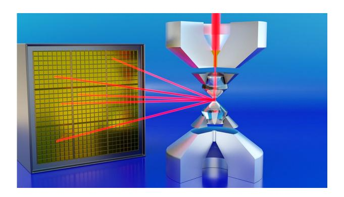
ORNL researchers used diamonds to compress materials to 1.2 million times ambient pressure and software to remove signal interference and extract data on pressure-induced atomic structures. Credit: Jill Hemman/ORNL, U.S. Dept. of Energy
