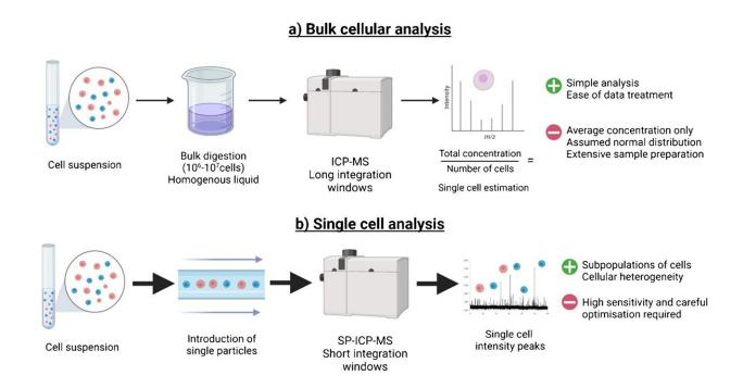
Comparison of main features of bulk solution ICP-MS and SP-ICP-MS for cellular analysis. Credit: *Analytical and Bioanalytical Chemistry* (2023). DOI: 10.1007/s00216-023-04721-8
