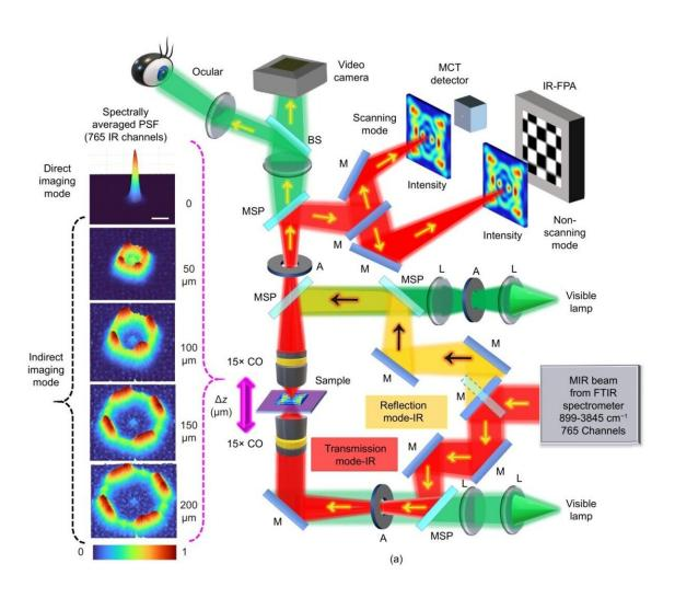
Figure 1. Schematic of IRM system at Australian Synchrotron. Credit: Compuscript Ltd
