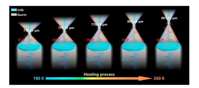
The working principle of CVBAM operating in 1.8–2.2 THz with tunable focal length from 736.25  $\mu$ m (NA = 0.62) to 861.02  $\mu$ m (NA = 0.56). Credit: *Journal of Science: Advanced Materials and Devices* (2023). DOI: 10.1016/j.jsamd.2023.100560
