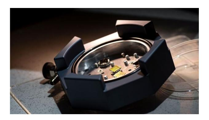
Tiny gold-coated silicon plates smaller than a fingernail are used as a printing surface. Credit: UOL
