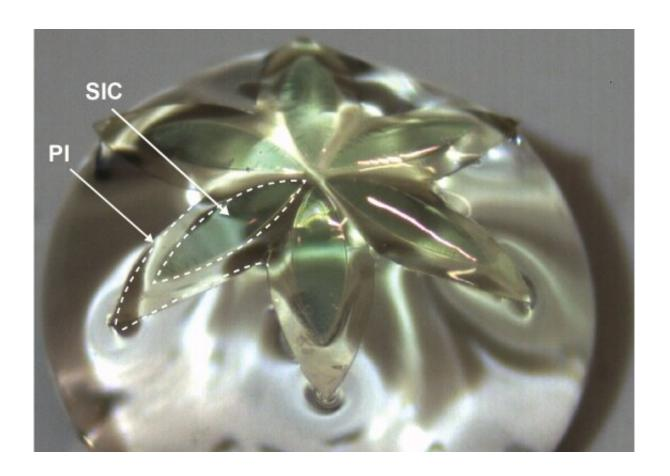
Optical image of an ultra-thin flower-shaped silicon carbide (SiC) wide bandgap semiconductor stamped onto a polyimide (PI) film and placed onto a water droplet. Credit: Thanh-An Truong
