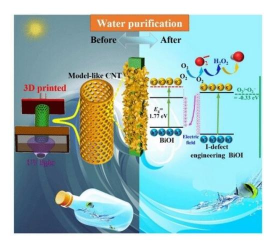
The scheme of in-situ photocatalytic film on 3D-printed polymer as an efficient purification application. Credit: IOCAS
