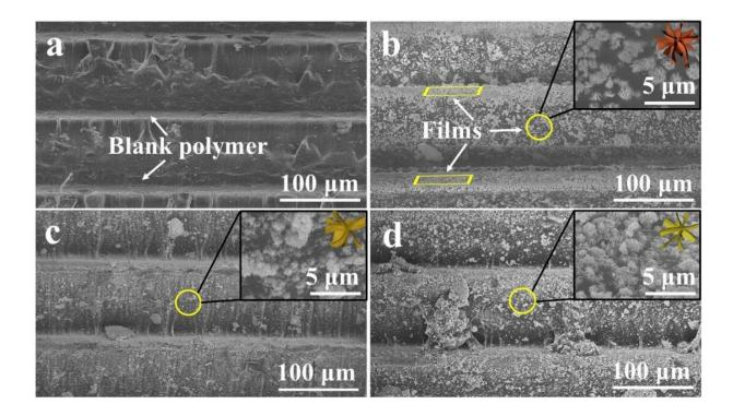
Scanning electron microscopy (SEM) images of (a) the blank polymer substrate and I-defect engineering films fabricated at (b) pH 2.48, (c) pH 4~6, (d) pH 6~9. Credit: IOCAS
