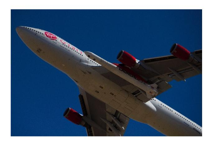
The Virgin Orbit 'Cosmic Girl' -- a modified Boeing 747 carrying a LauncherOne rocket under its wing -- takes off from Mojave Air and Space Port in 2021.
