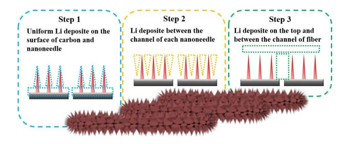
Bottom—up uniform Li deposition behavior realized by unique three—dimensional nanoneedle arrays. Credit: *Journal of Energy Chemistry* (2022). DOI: 10.1016/j.jechem.2022.10.023
