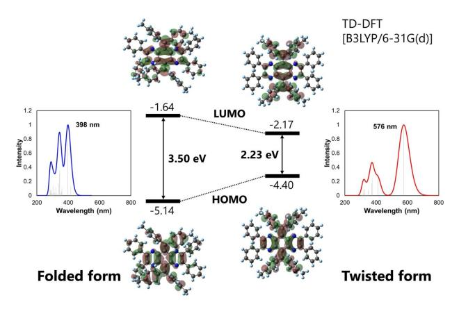
The folded and twisted isomers absorb different wavelengths of light. Credit: *Materials Chemistry Frontiers* (2023). DOI: 10.1039/D2QM01199A
