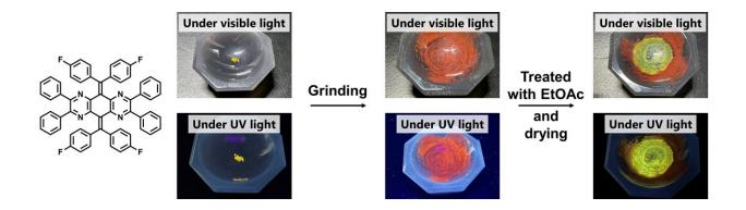
When ground into amorphous solid and treated with appropriate solvents the light absorption and emission changes. Credit: *Materials Chemistry Frontiers* (2023). DOI: 10.1039/D2QM01199A
