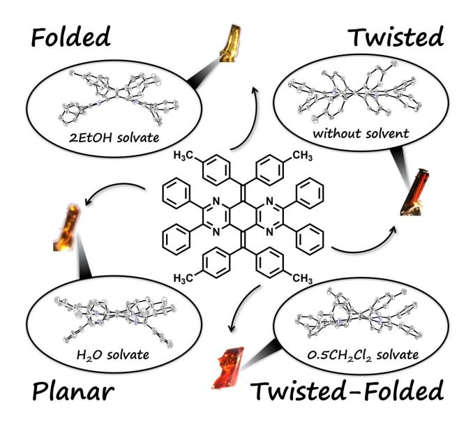
The methyl derivative of the new compound has four different isomers, with different crystal structures each. Credit: *Materials Chemistry Frontiers* (2023).
