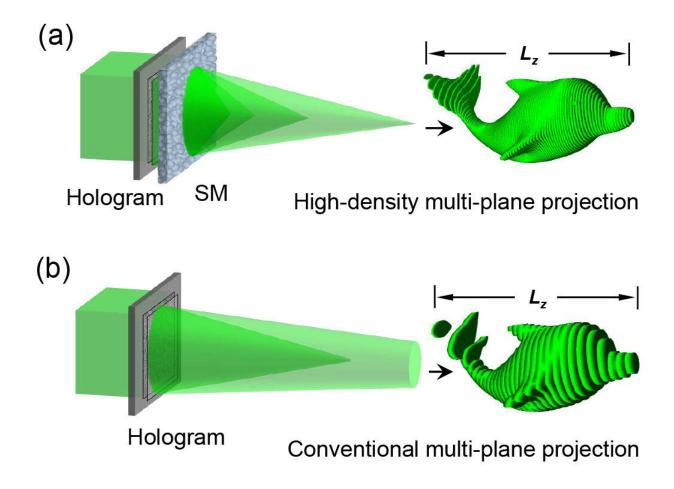
The new 3D scattering-assisted dynamic holography approach creates a digital hologram by projecting high-resolution images onto planes spaced closely together (a), achieving a more realistic representation than conventional holography techniques (b). Credit: Lei Gong, University of Science and
