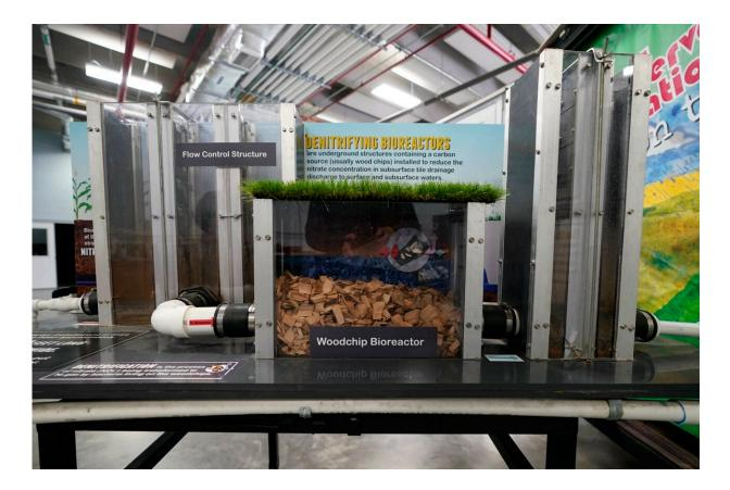
A bioreactor model is seen during an edge-of-field workshop at the Ames Water Treatment Plant, Thursday, March 2, 2023, in Ames, Iowa. Simple systems called bioreactors and streamside buffers help filter nitrates from rainwater before it can reach streams and rivers. Credit: AP Photo/Charlie Neibergall
