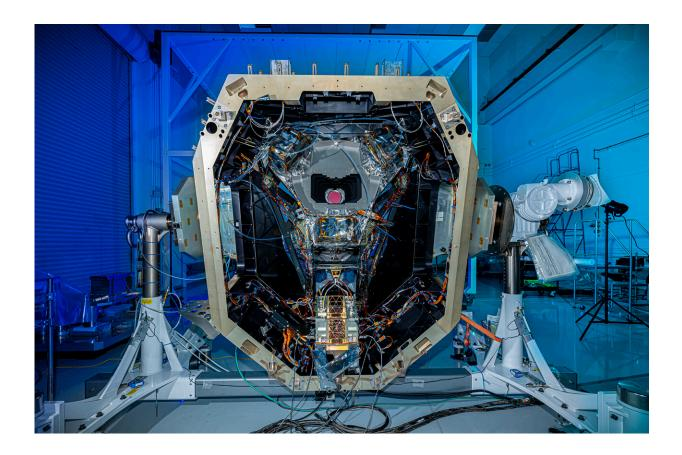
This photo shows the Roman Space Telescope's Cold Sensing Module, which contains the Simplified Relative Calibration System (sRCS). Credit: Ball Aerospace
