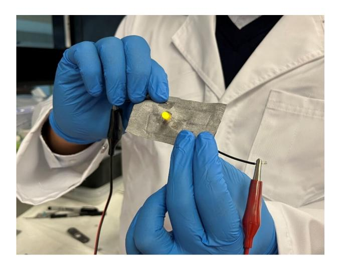
The fabric becomes conductive when coated with with a special "breathable" metallic layer. Credit: Flinders University
