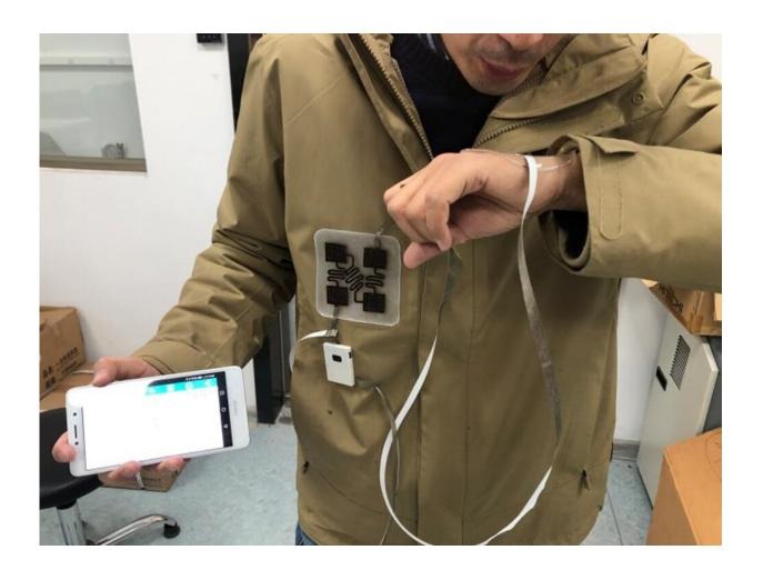
A Penn State-led research team developed a standalone system to monitor nitrogen dioxide in exhaled breath and in the environment. Fabricated from the same nanocomposite material, the self-powered system stretches to adhere to skin or clothes. Credit: Provided by Huanyu "Larry" Cheng/Penn State
