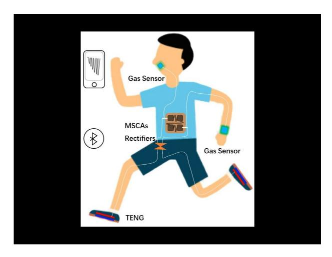
The standalone system converts energy from human movement, like running) to power gas sensors at the mouth and wrist, as well as to send data via Bluetooth. Credit: Provided by Huanyu "Larry" Cheng/Penn State
