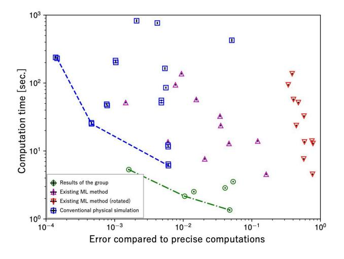
Comparison of computation time and errors from the ground truth. The fast and accurate prediction is represented by the bottom left part of the figure. The proposed method (green) achieves a favorable speed-accuracy tradeoff that cannot be obtained with conventional physical simulation (blue) or existing machine learning models proposed by Brandstetter et al. [ICLR 2022] (magenta and red). Credit: Masanobu Horie
