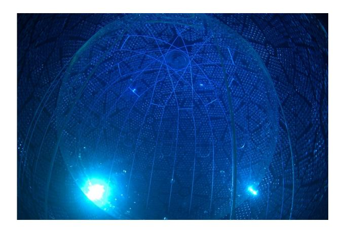
A picture taken using the team's PSUP mounted cameras in 2017, when the detector was full of water. Credit: The SNO+ Collaboration.
