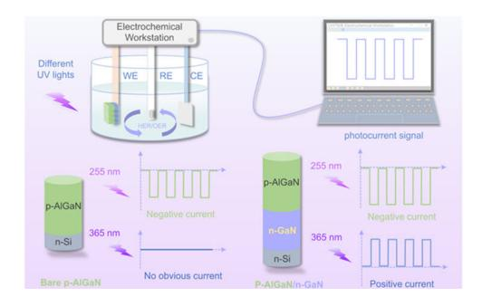
Working diagram, working mechanism, and photocurrent signal of the p-AlGaN/n-GaN based PEC UV PD under different wavelengths. Credit: Wang et al / NJUPT
