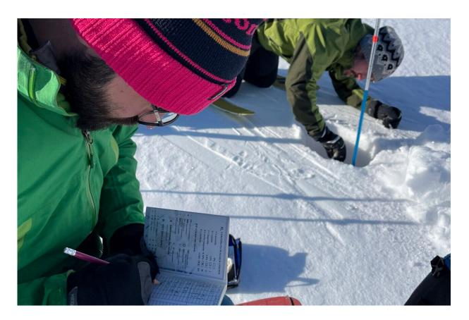
Carlo Marin, remote sensing engineer and test manager, notes the results of the 7 measurements taken at each point. In the background Riccardo Barella measures the temperature in a small hole. The temperature is taken at two different depths 10cm and 30cm and always from the the side not hit by the sun so that the results remain as consistent as possible. Credit: Eurac Research | Maurizio Gretter
