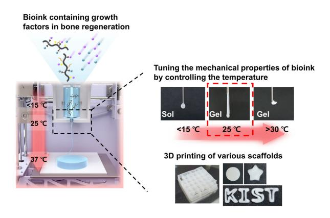
Tuning mechanical properties of bioink according to temperature and 3d scaffold printing. Credit: Korea Institute of Science and Technology
