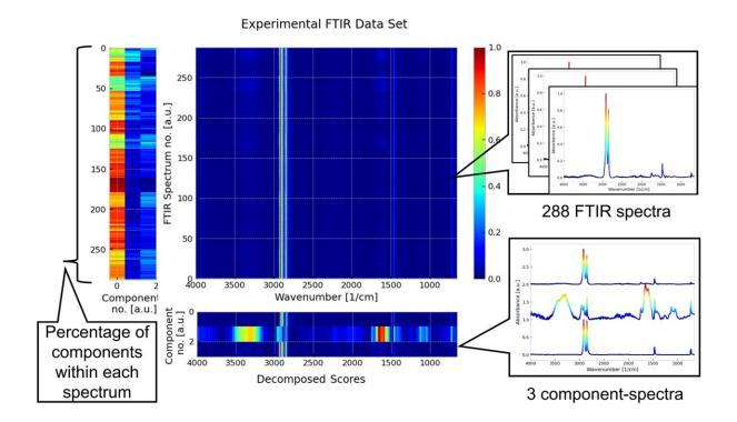
Principle of the multivariate analysis of a set of FTIR spectra. The color scale corresponds both to the intensity and the percentage of HDPE and the extractables (odorants, impurities). Credit: Fraunhofer LBF
