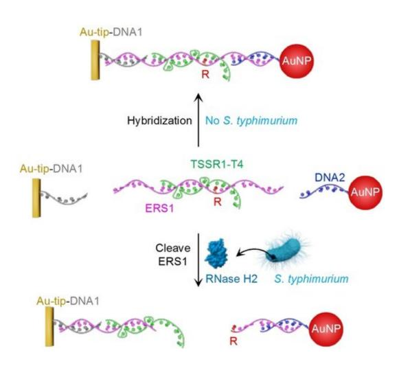
A simple and portable Au-on-Au tip sensor was constructed to achieve specific, sensitive, and colorimetric detection of Salmonella typhimurium using an RNase H2-specific nucleic acid molecule derived from a random-sequence synthetic nucleic acid pool by in vitro selection. Credit: *Angewandte Chemie International Edition* (2023). DOI: 10.1002/anie.202300828
