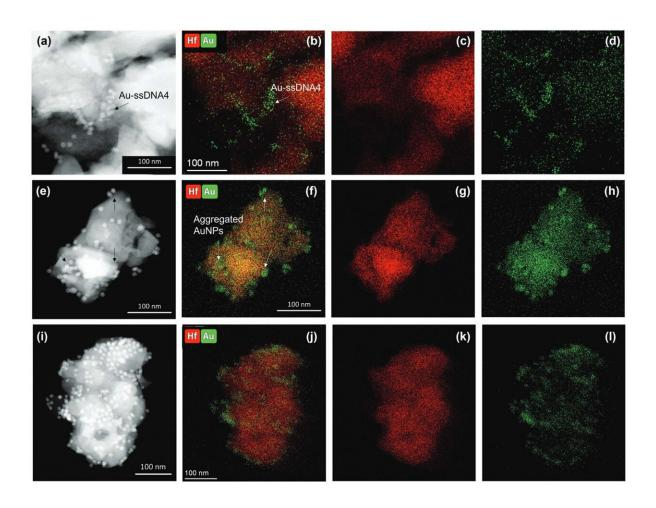
The nano-assembly mpox rapid test before (a) and after (e) the addition of mpox DNA. The red and green color encodes for gold nanoparticles and hafnium disulfide nanoplatelets respectively. The white arrows show dispersed gold nanoparticles and grouped gold nanoparticles. Credit: Dipanjan Pan
