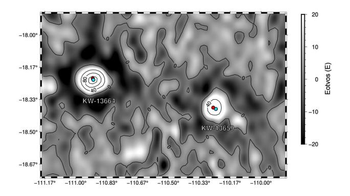
Two seamounts from the Kim-Wessel catalog before and after being centered (20 Eotvos contours). Light blue colored points indicate the original location of the seamounts. Red points are the new centers chosen based on the maximum VGG value. Credit: *Earth and Space Science* (2023). DOI: 10.1029/2022EA002331
