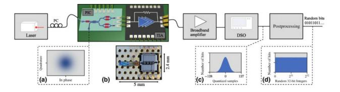
An overview of the QRNG setup. (a) The vacuum noise that is used as a source to generate random numbers. (b) A micrograph of the manufactured PIC and TIA. (c) The Gaussian distribution after digitization. (d) The distribution of the distilled random 32-bit integers, grouped into 256 bins. Credit: *PRX Quantum* (2023). DOI: 10.1103/PRXQuantum.4.010330
