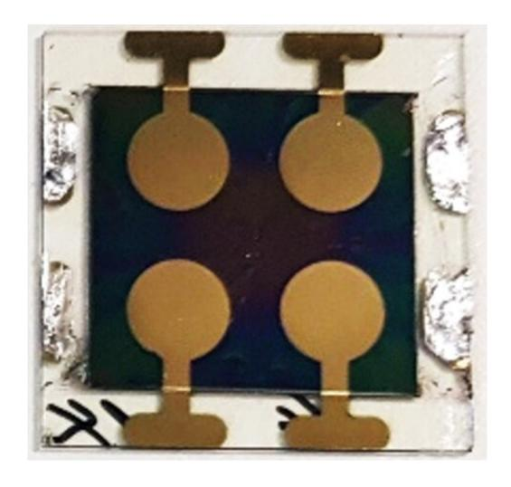
An image of a thin film multi-energy X-ray detector device. Credit: Exciton Science
