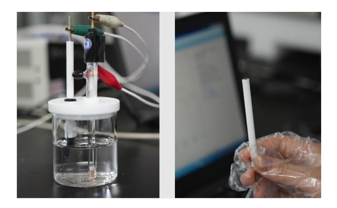
Portable Electrochemical Sensor Designed for Lead Ion Detection. Credit: Journal of Electroanalytical Chemistry (2023). DOI: 10.1016/j.jelechem.2023.117320
