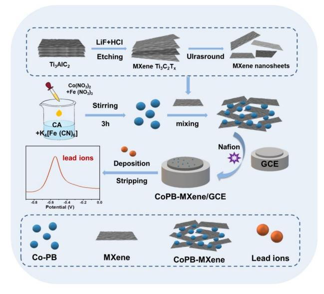
Schematic preparation process of the sensor and electrochemical detection of Pb<sup>2+</sup>. Credit: *Journal of Electroanalytical Chemistry* (2023). DOI: 10.1016/j.jelechem.2023.117320
