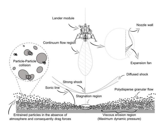
Near-field plume-surface interaction and regolith erosion and dispersal during the lunar landing. Credit: Reproduced with permission from A. Rahimi, O. Ejtehadi, K.H. Lee, R.S. Myong, Acta Astronautica, 175 (2020) 308-326. ©2018 Elsevier.
