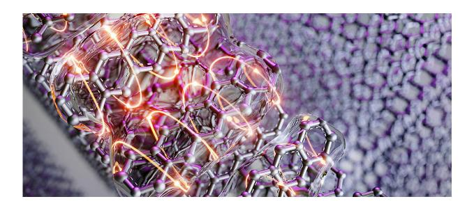
Illustration of exciton splitting in the organic semiconductor pentacene, which consists of five benzene rings each. Instead of the usual two free charge carriers, absorption of a photon in pentacene generates four free charge carriers, represented by orange tracks. Credit: TU Berlin
