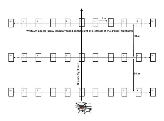
Illustration of the experimental layout of spray cards for establishing optimum droplet density by spraying at different heights using an Agras T20 drone fitted with a Micronair 12 ultra-low volume (ULV) spraying boom. Credit: *Drones* (2023). DOI: 10.3390/drones7040233
