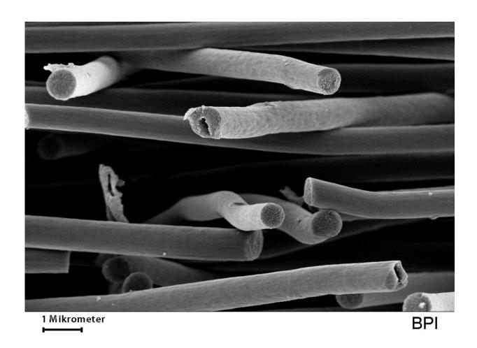
Scanning electron image of fibers in a novel electrospun nonwoven which exhibits an unusual combination of high electrical conductivity and extremely low thermal conductivity. Credit: UBT
