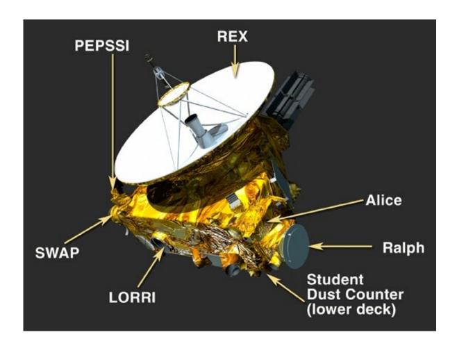
The New Horizons instrument payload that is currently doing planetary science, heliospheric measurements, and astrophysical observations. Credit: NASA/Johns Hopkins University Applied Physics Laboratory/Southwest Research Institute
