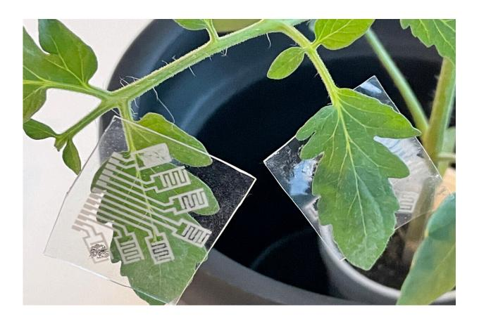
Researchers from North Carolina State University have developed an electronic patch that can be applied to the leaves of plants to monitor crops for different pathogens – such as viral and fungal infections – and stresses such as drought or salinity. In testing, the researchers found the patch was able to detect a viral infection in tomatoes more than a week before growers would be able to detect any visible symptoms of disease. Credit: Qingshan Wei, NC State University
