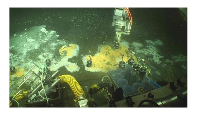
Remotely operated vehicle (ROV Jason) takes samples of hydrothermal microbial mat 2000m below sea level in the Guaymas Basin, Mexico. Credit: Peter Girguis and E/V Nautilus
