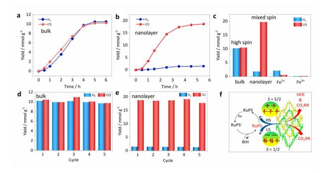
Catalytic performance. Time-dependent H2 and CO yield with (a) HS bulk and (b) MS nanolayer o-1. (c) H2 and CO yields through HS bulk o-1, MS nanolayer and control samples as catalysts after 4 h irradiation. Recycle experiments for H2 and CO production with (d) HS bulk o-1 and (e) MS nanolayer o-1 as catalysts. (f) Proposed photocatalytic mechanism in this work. Credit: WU Dayu
