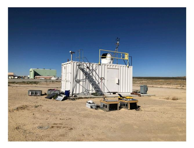
Portable solar spectrometers measuring alongside a higher resolution solar spectrometer. Researchers performed side-by-side measurements before and after field campaigns to ensure instrument stability and check data quality. Photo taken at NASA's Armstrong Flight Research Center in Edwards, California. Credit: Frausto-Vicencio/UCR
