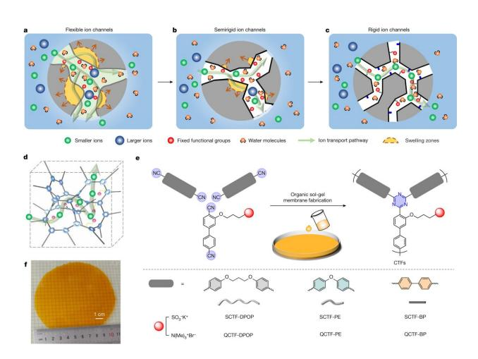
Schematic illustrations showing existing and proposed ion-selective polymer membranes with varying ion channels. a, Membranes with flexible ion channels. These contain microphase-separated morphology derived from the assembly of hydrophilic ion-conductive moieties and hydrophobic flexible-polymer backbones, represented by Nafion. b, Ion-selective microporous membranes with semirigid ion channels. The channels are formed by intrinsic micropores
