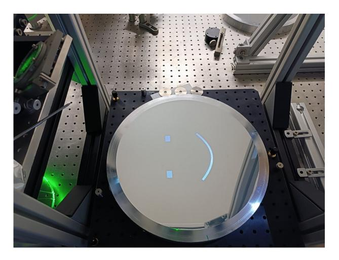
The researchers created the mirrors by using chemical vapor deposition to grow membrane mirrors on a rotating liquid inside a vacuum chamber. This allowed them to form parabolic thin membrane that can be used as the primary mirror of a telescope once coated with a reflecting surface such as aluminum. Credit: Sebastian Rabien, Max Planck Institute for Extraterrestrial Physics
