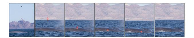
Photo sequence showing DTAG deployment using the drop system, and the release of tag holder and fins on impact that float for recovery and reuse. Credit: *Royal Society Open Science* (2023). DOI: 10.1098/rsos.221376
